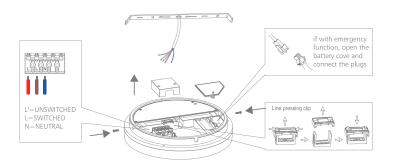
Remove the driver cover and line pressing, connect the wires correspondingly. (If emergency function, open the battery cove and connect the plugs). Then Switch
