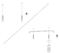
Knock the plastic anchor into ceiling and fix bracket with screw into the ceiling.
